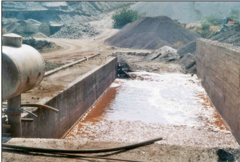
Figure 3.49: Dewatering of tailings in concrete basins [110, IGME, 2002]
