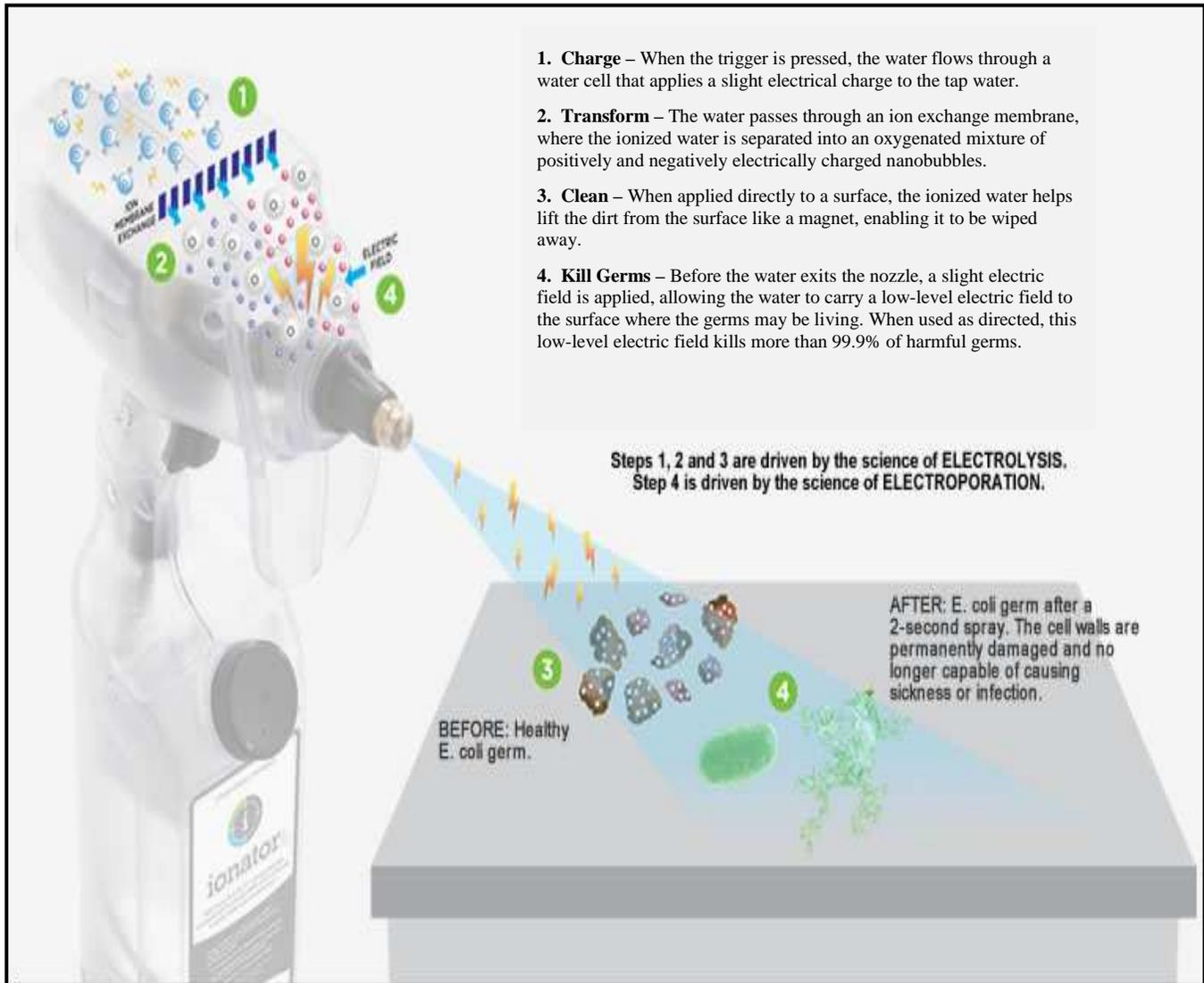
**Figure 1. The science inside the Ionator.** Two key scientific concepts drive the technology in the Activeion products: electrolysis and electroporation. The science of electrolysis is over 100 years old, and the science of electroporation has been around for decades. (Diagram courtesy of Activeion Cleaning Solutions, LLC., Copyright © 2010, <http://www.activeion.com/science/default.aspx>.)
