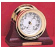
**Barometers** - A barometer is an instrument used to measure pressure in the atmosphere that contains liquid mercury. A Bourdon tube gauge is an alternative to mercury-containing barometers.
