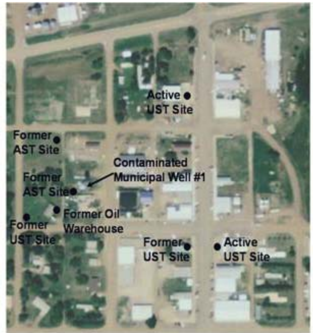
Historic and Current Petroleum Sites in Timber Lake demonstrates numerous potential contamination sources
