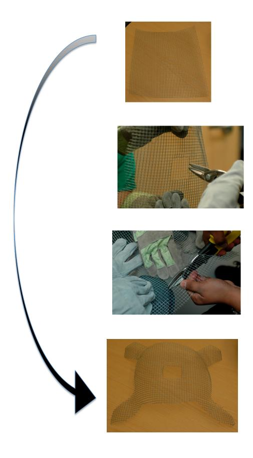
Once you have finished cutting out the mesh portion of your dust trap, set it aside. *Note:* If you are making multiple dust traps, it can be helpful to use the first mesh cut-out as a template for the remaining mesh cut-outs.
