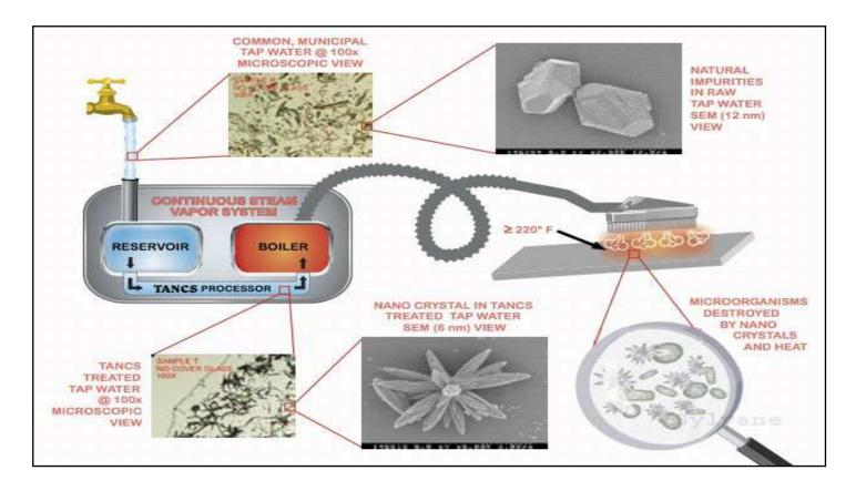
Figure 2. Thermal Accelerated Nano Crystal Sanitation Steam Vapor System. (Diagram courtesy of Sylvane, Inc., Copyright © 2010, http://www.sylvane.com/learning-center/tancs.html.)
