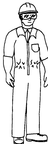
LEVEL D Protection Basic work uniform, i.e., long-sleeve coveralls, gloves, hardhat, boots, faceshield or goggles.
