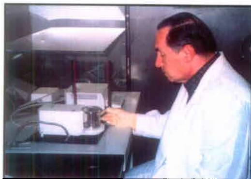
Carl Palumbo, Gravimetric Laboratory Analyst, CIE, weighing a PM 2.5 filter for participating tribes.
