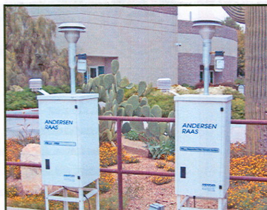
TAMS PM2.5 Particulate Samplers located on the University of Nevada-Las Vegas campus.
