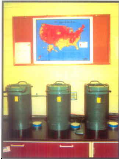
Charcoal canister analytical system. These canisters are part of an 8 station system designed to measure radon concentration from 4 inch diameter barrier face charcoal canisters.
