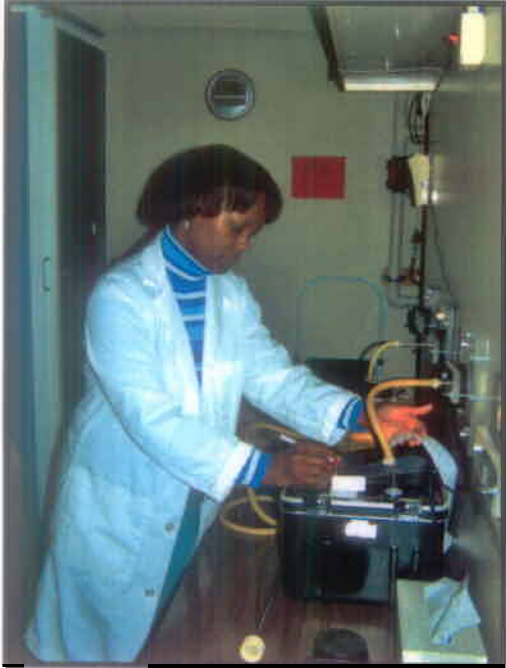
Evelyn Clay is servicing a commercially available radon detector that is being used to survey the area outside of the environmental radon chamber .
