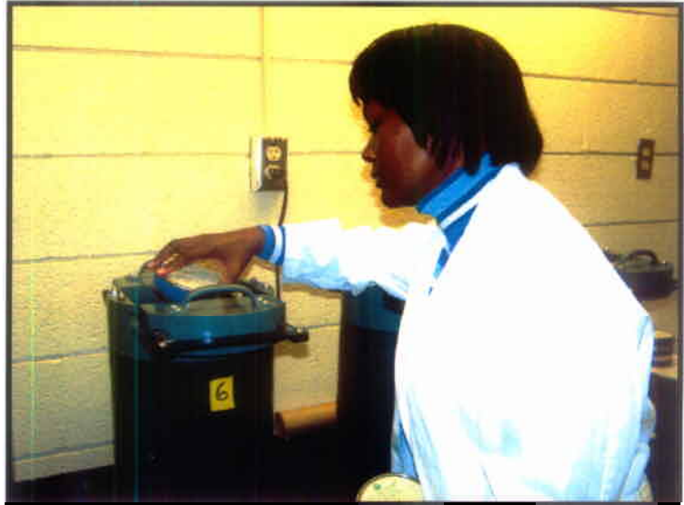
In this photo, Evelyn Clay is inserting a charcoal canister into one of the stations in the charcoal canister analytical system.
