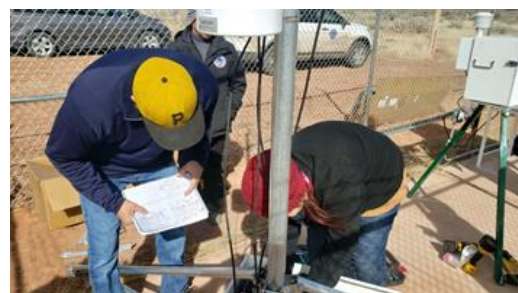
Mike King (TAMS), Henry Gerard (USEPA), and Kaelyn Morgan (NNEPA) connecting meteorological equipment to a datalogger.
