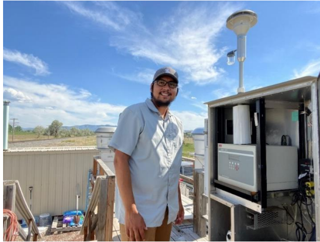
Keith Moore, Air Quality Technician for the Shoshone-Bannock Tribe's Air Quality Department, stands next to their BAM-1020 particulate monitor located on the Fort Hall Reservation in Southeastern Idaho.
