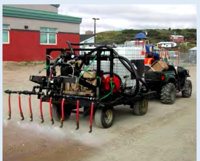
Portable applicators for spraying dust suppressants can be easily flown to rural Alaska on a small aircraft. The system can be mounted to a trailer and pulled by an ATV. (Photo from UAF/ADOT&PF report: “Managing Dust on Unpaved Roads and Airports”)
