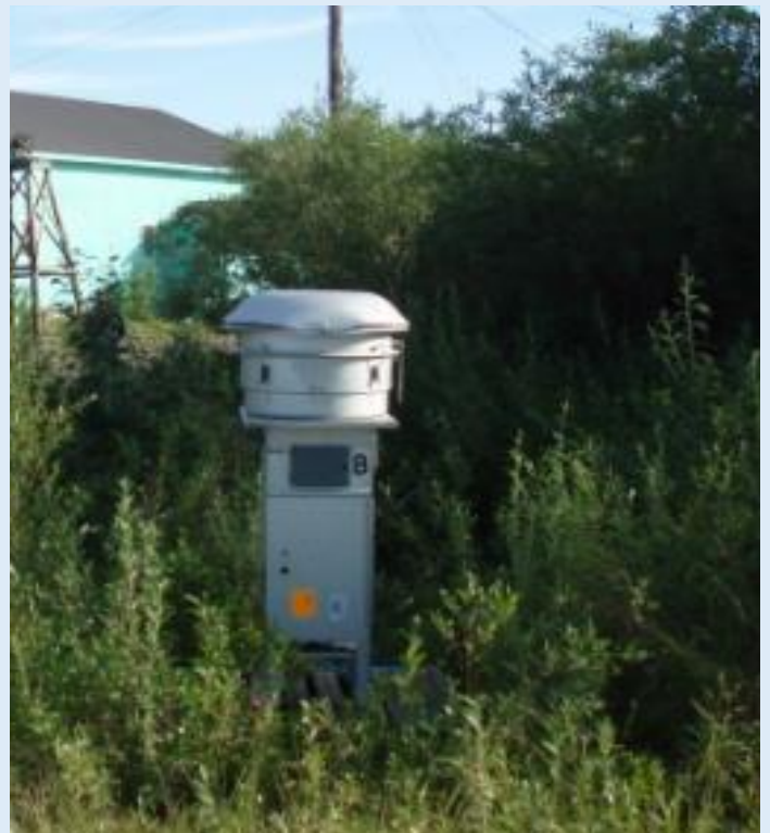
Stationary air monitors can be placed alongside unpaved roads in communities near a reliable power source and frequently-used routes where the most individuals are expected to be exposed to dust. Photo credit: Noorvik (2012)
