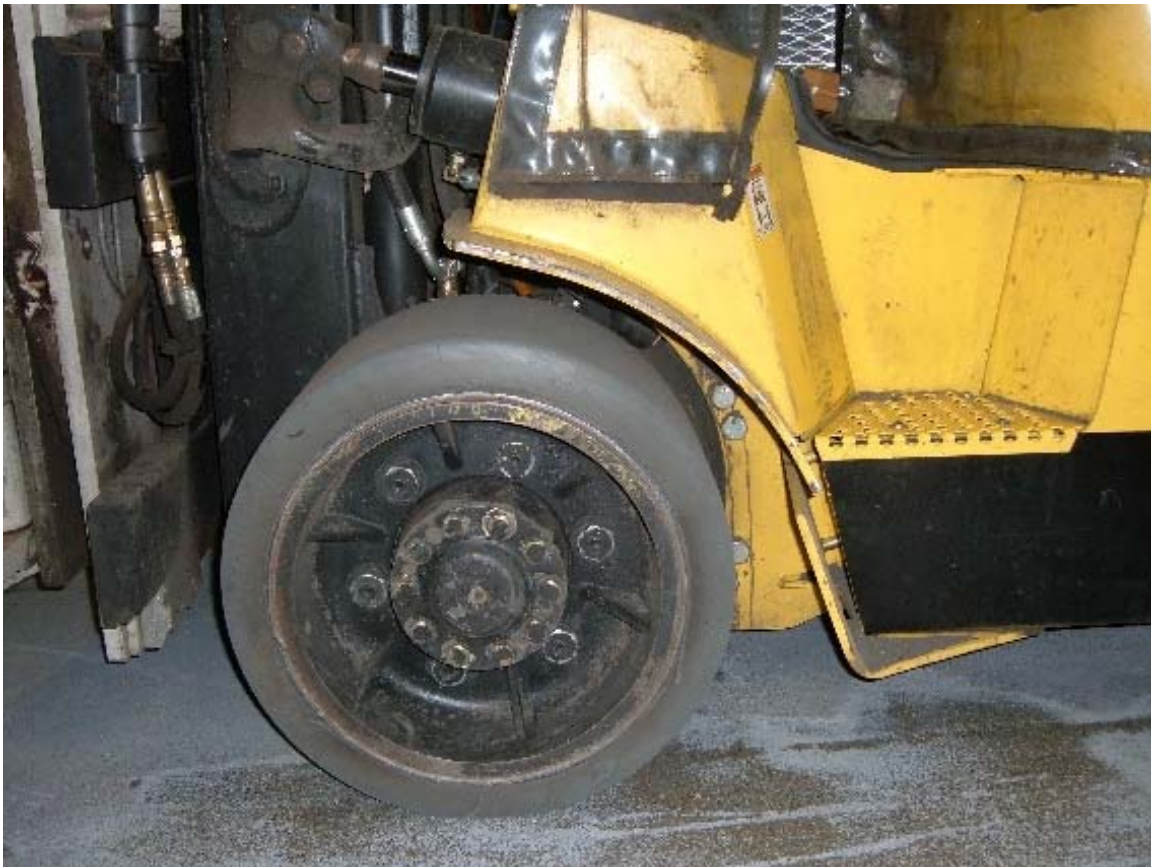
Fork lift tires can be a large source of tire dust. The tires rub and release dust when making tight turns.
