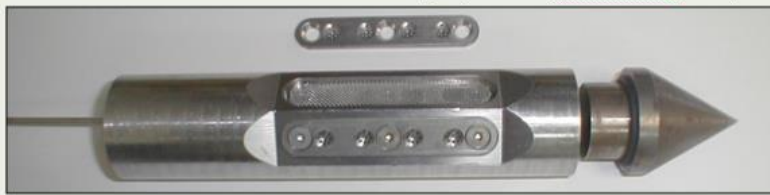
Waterloo Advanced Profiling System (Waterloo APS™)
