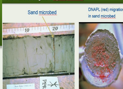
Structure and Pore Fluids Intact 9 x 9 m Cell DNAPL Migration in Aquitard Microbeds
