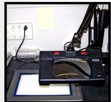
Light Table Magnification used to search for filter defects
