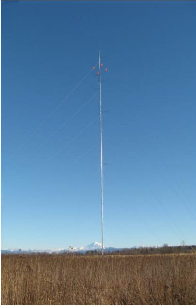
Installed Anemometer Tower on Lummi Reservation. Source: Jeremy Freimund, Lummi Nation Water Resource Division Manager
