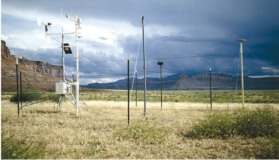
USGS meteorological station established to monitor climate (temperature, precipitation, wind direction and strength) and geologic processes (erosion and deposition) for studies of land use and landscape change on the Colorado Plateau (USGS Earth Surface Dynamics Program, http://climweb.cr.usgs.gov/info/sw/clim-met/ ). San Juan County, Utah. Photograph by Rich Reynolds, USGS.
