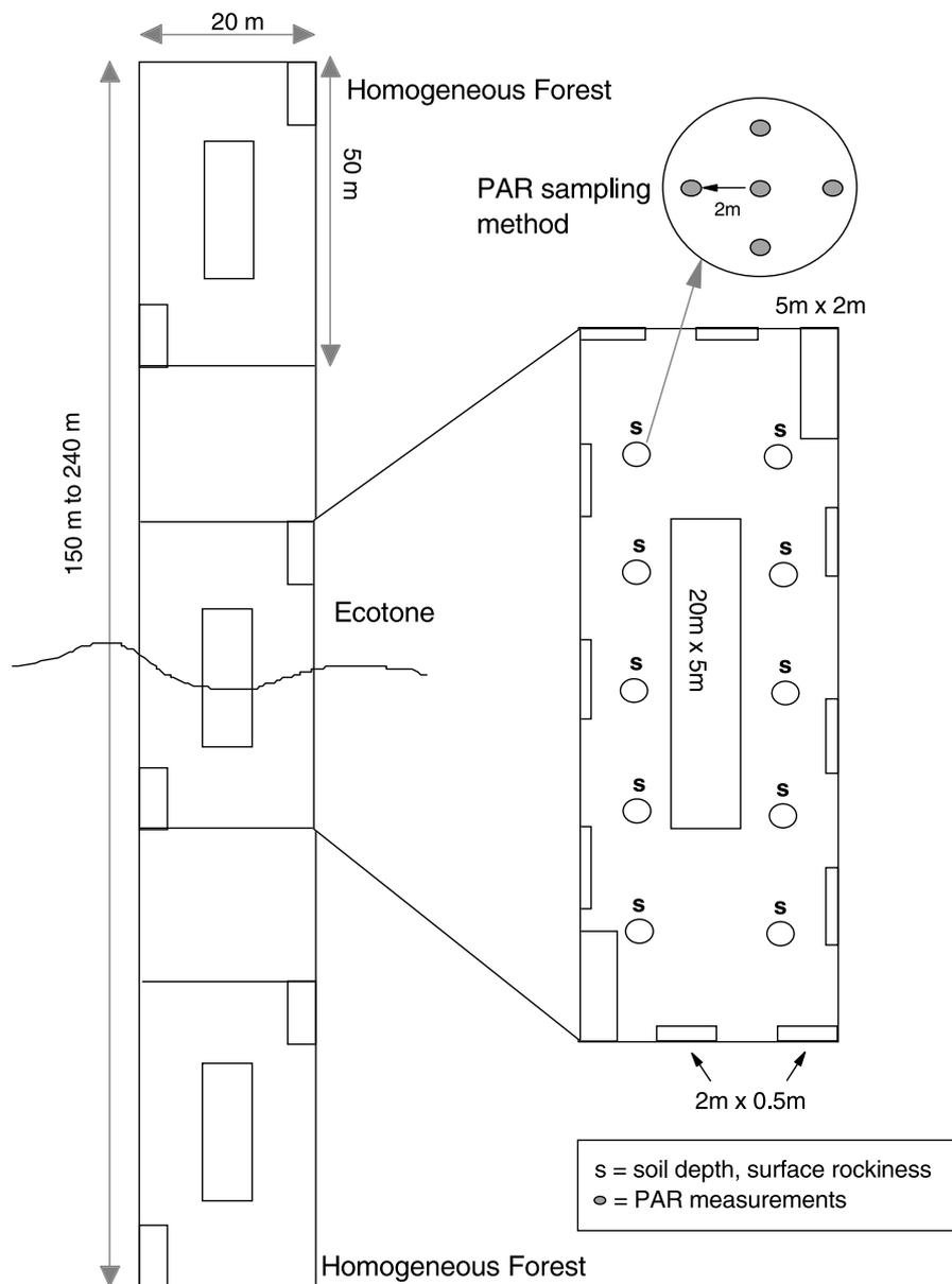
Figure 1. Diagram of transect, plot layout, and methods.
